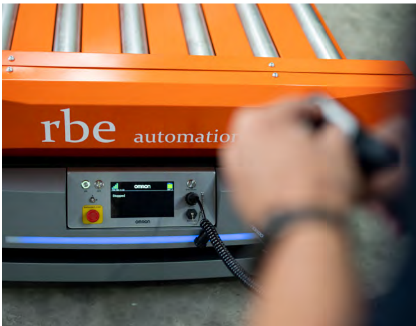
Above: Automatic pallet or bin mover by RBE Hortworx. Photo: Tom Allan
